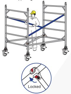
Locate the platform on the top rung of the 5-rung frame. Ensure that 4. the scaffolding is correctly aligned by using a spirit level.
